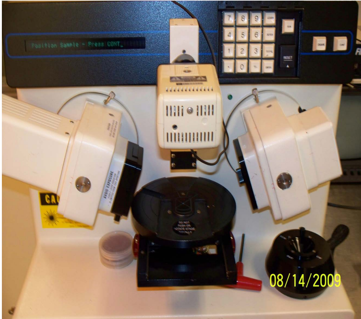
Figure 2.2: Ellipsometer Used to Measure the Thickness of the Silicon Nitride Film
