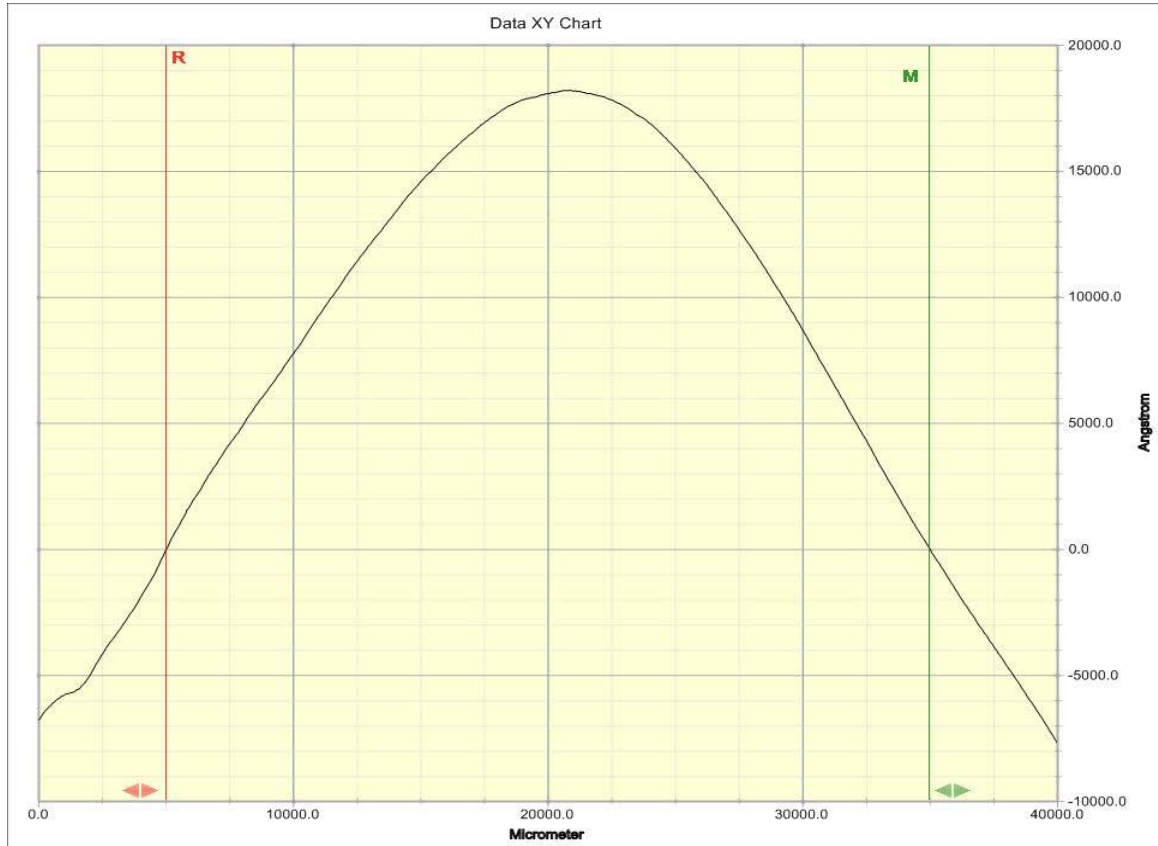
Figure 2.5: Scan of a Wafer before Deposition of Silicon Nitride
