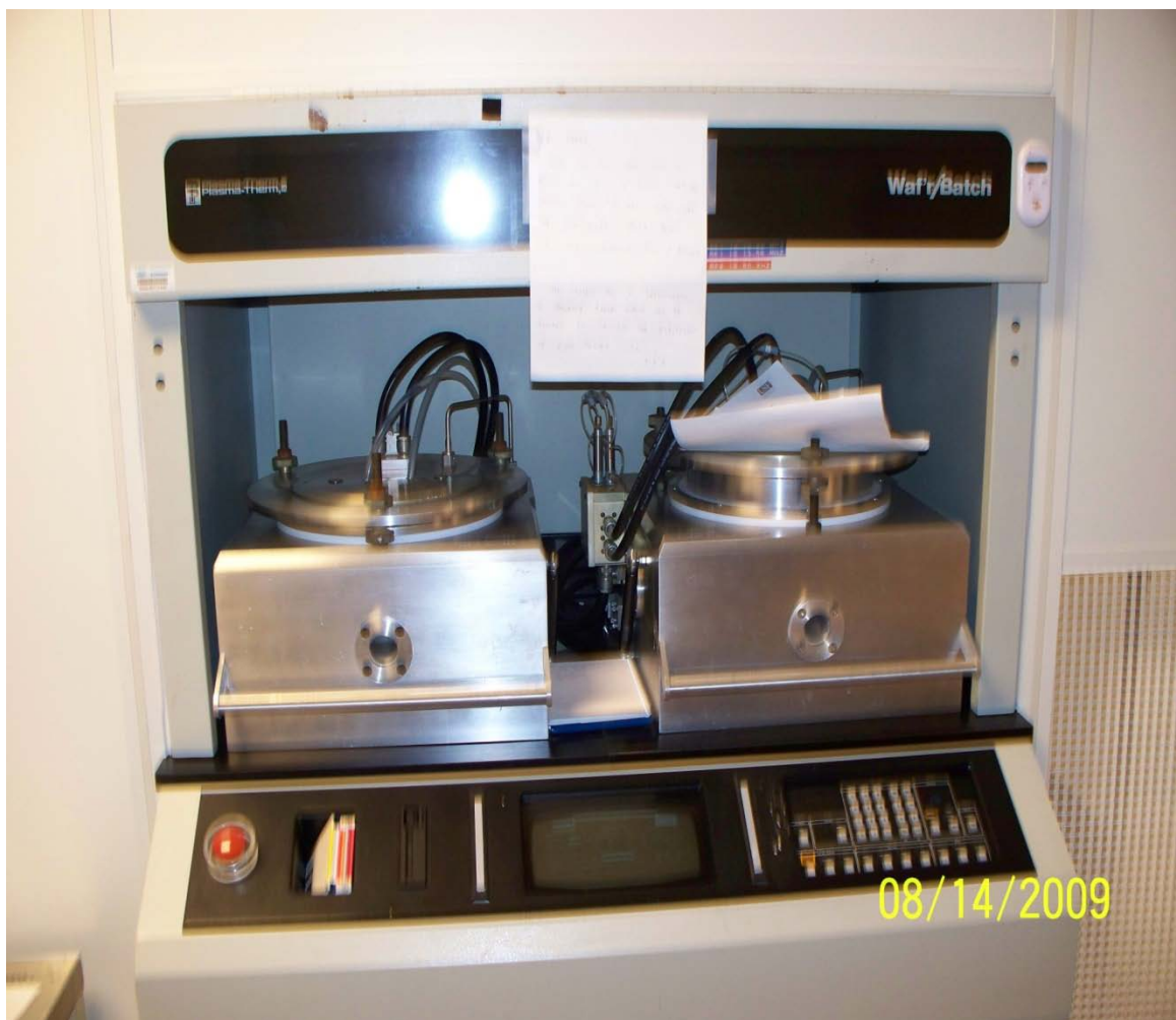
Figure 2.1: Plasma Enhanced Chemical Vapor Deposition (PECVD) System Used to Deposit and Characterize Silicon Nitride Thin Film
