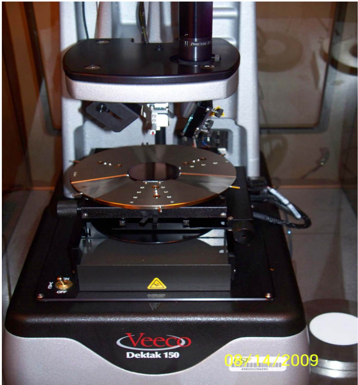
Figure 2.3: Surface Profilometer Used to Measure the Curvature in the Silicon Substrate and Compute the Film Stress
